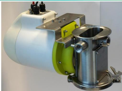
Figure 3: Eyecon mounted on Hosakawa Alpine Mill Integration
